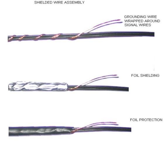
A good and cost effective way to shield wire is as such. (Shown in the figure above)
