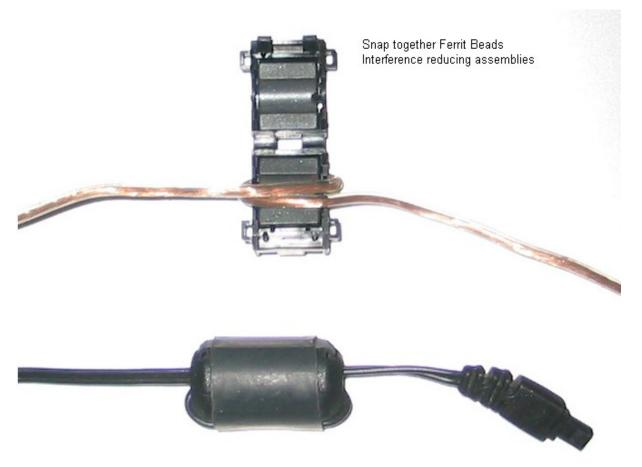
Alternative methods to reduce interference includes purchasing a ferrite bead and wrapping the ignition and ancillary device signal wires around the ferrite bead. This is a common and effective way to remove interference from the source. Typical ferrite beads can be found on many small electrical device power wires such as vehicle after market stereos, camera's, computer monitors etc.
