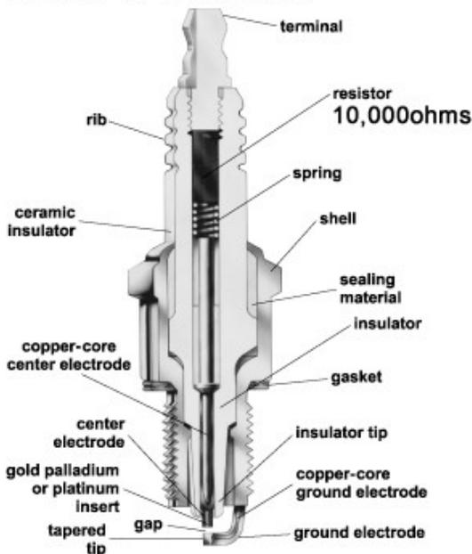
*LEFT, an internal picture of a standard spark plug. Typically a carbon resistor is used to reduce EMI and RFI interference levels in the vehicle. It should be noted that WeaponX spec'd spark plugs use a solid OFC core allowing for a zero ohm plug.*
