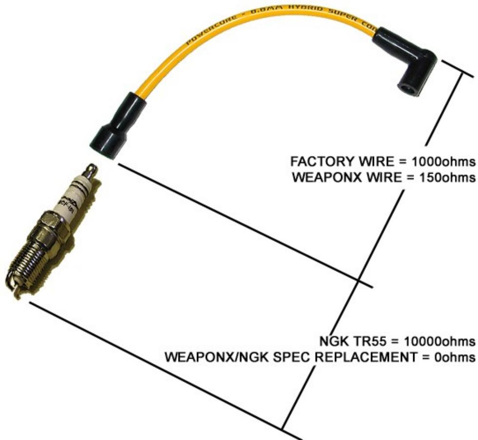
**TOTAL FACTORY RESISTANCE IN THE IGNITION CIRCUIT 11,000ohms**
