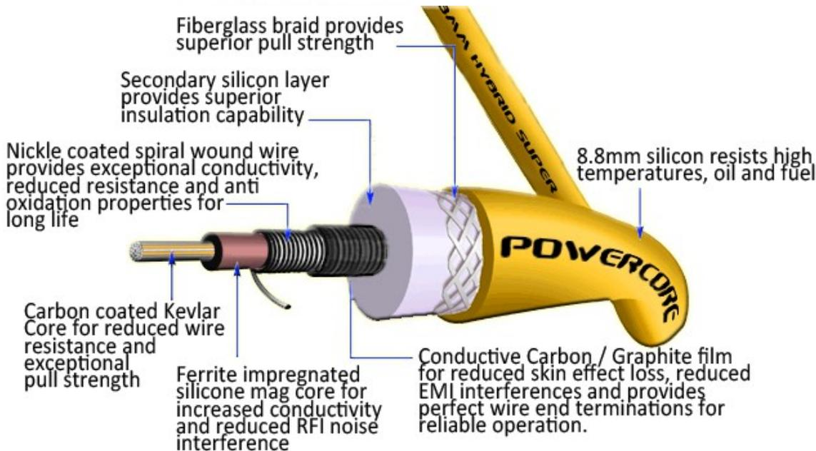
The PowerCORE 8.8mm wire uses a graphite skin over the spiral wound conductor. While it adds additional cost to the wire, this has several performance advantages.
