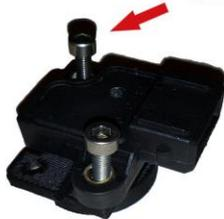
*The ignition module can be assembled with or without the heatsink assembly. For a lower profile mount the ignition module amplifier with the metal surface facing downwards and with the connector facing the closed portion of the coil adaptor.*
