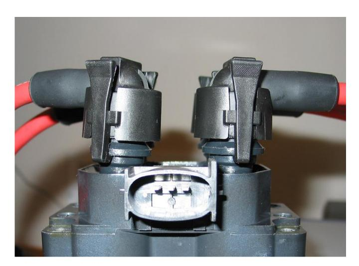
Notice all the clasps are FIRMLY sitting on the towers with a proper installation.
