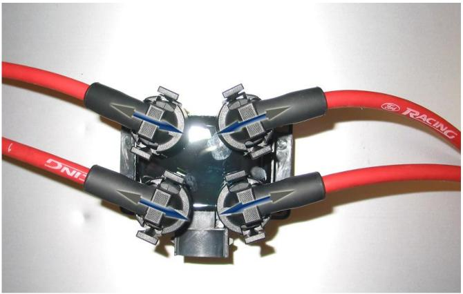
terminal the spark plug wire is not properly seated in the high retention / high output brass terminal.
